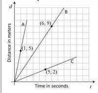
Solution: Carli is correct. Whenever the ratio between two quantities is constant, the graph of the relationship between them is a straight line through (0,0). We can also say that for each robot, the relationship between the time and distance is a proportional relationship.
